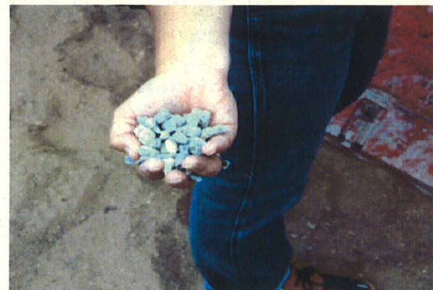
Bentonite material used for well plugging.
